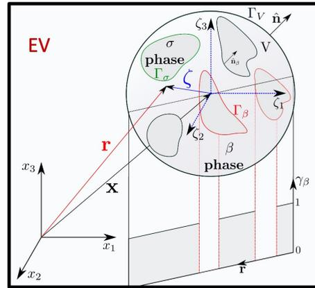
To consider both phases in the same computational domain, one must account for the multi-scale aspects of porous media structures. **One must locally average the governing equations using Volume Average Navier-Stokes (VANS) equations<sup>[10]</sup> over a volume that might contain n-phases.**
