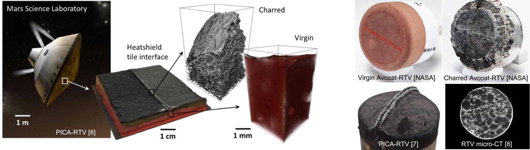
Current tiled ablative heatshields use Room Temperature Vulcanizing (RTV) silicone as a gap filler between tiles. Fences are formed between tiles during ablation impacting the environment.
